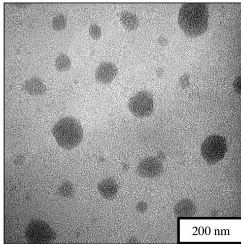
**Figure 1:** Morphology of NLC-ZZ formulation A1 observed under transmission electron (magnification of 150 000).
