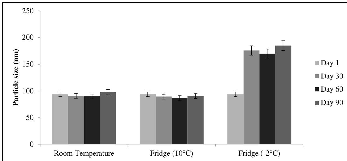
**Figure 2:** NLC-ZZ formulation A1 stability based on particle size observed for 90 days in storage at room temperature, 10°C, and -2°C. Data presented in mean  $\pm$  standard deviation (SD) (n=3).
