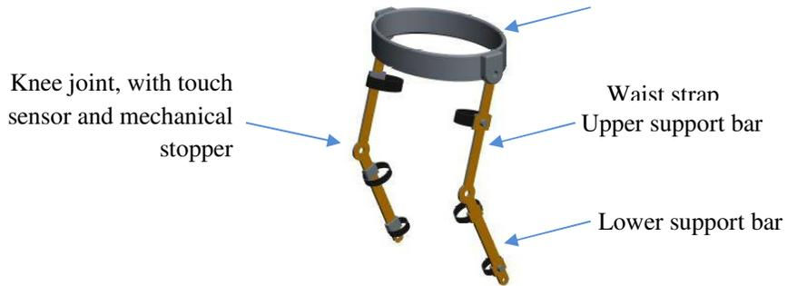
**Figure 4:** The wearable leg brace
