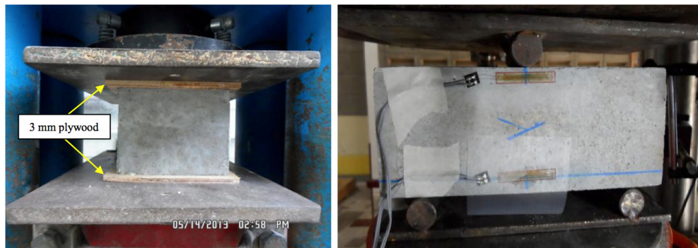
Figure 2: (a) Compression test for CPB specimen, (b) Flexural test for CPB specimen
