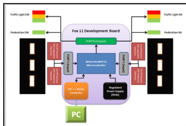
Fig. 5. System Block Diagram
