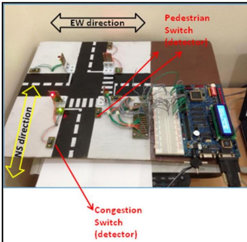
Fig. 8. 68HC11 Sequence Base Traffic Control System
