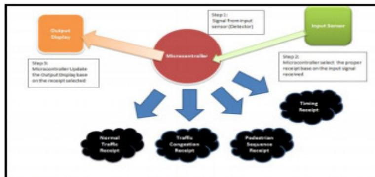
Fig. 3. System Methodologies – Sequence Base Method
