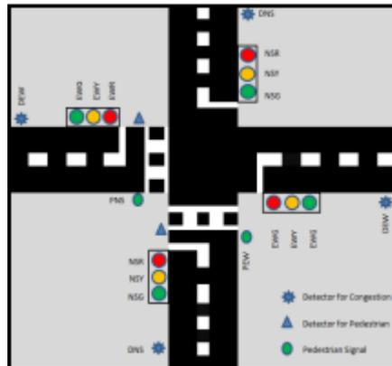
**Fig. 1.** Layout of the proposed traffic control system
