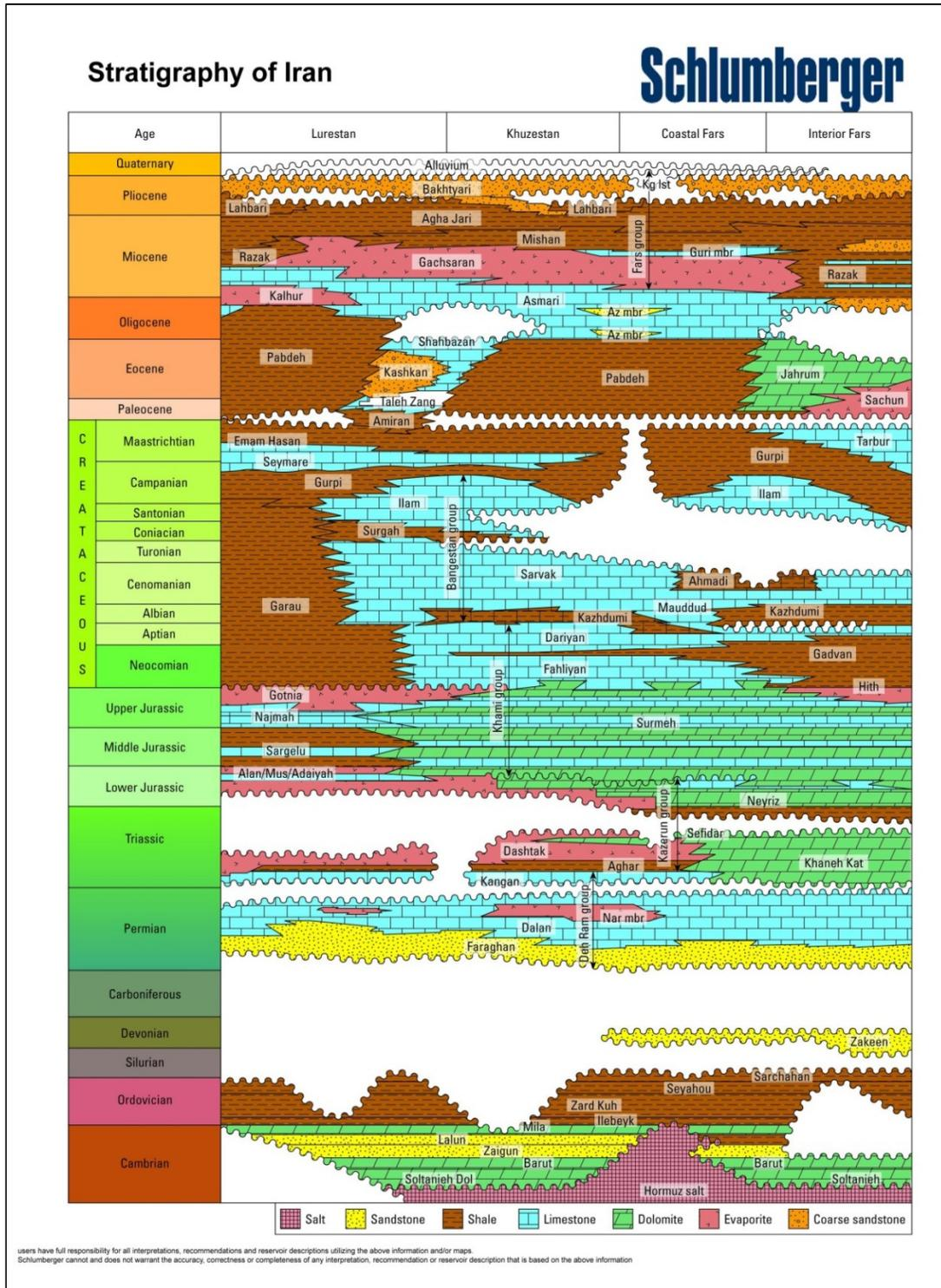
**Figure 2:** The location of Gachsaran oil field overlying the Asmari, Pabdeh, Gurpi and other reservoirs, and stratigraphic nomenclature of rock units and age relationships in the Zagros basin [3]
