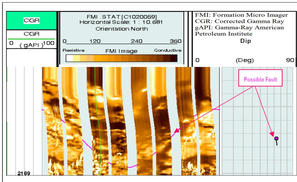
**Figure 4:** Close-up view of the possible fault
