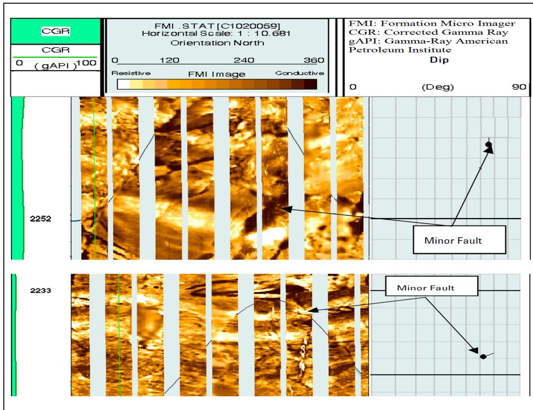
**Figure 5:** Close-up view of the two minor faults
