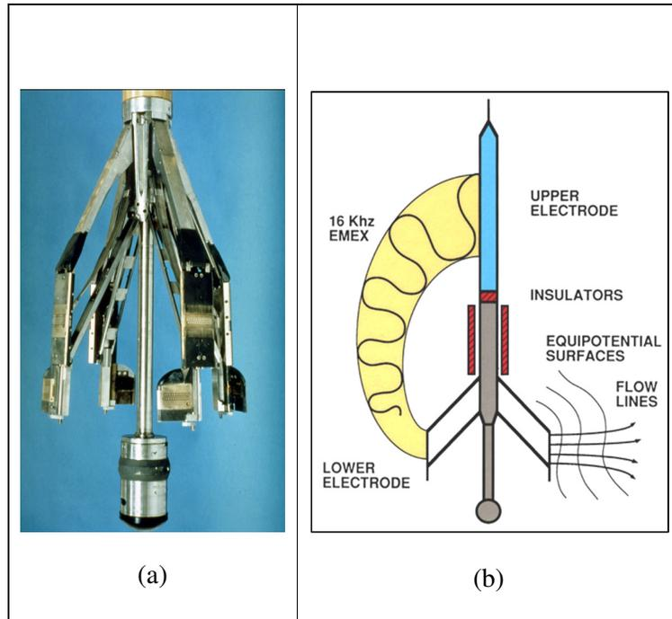
**Figure 3:** (a) Picture of an FMI tool and (b) explanation of the principle of measurement. EMEX current flows into the formation from the FBCC (upper electrodes) housing to the pad section (which is the FMI sonde section carrying 192 imaging microelectrodes), known as lower electrode.
