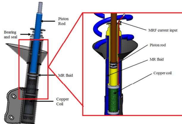
Fig. 1. Sectional view of the new design [4]
