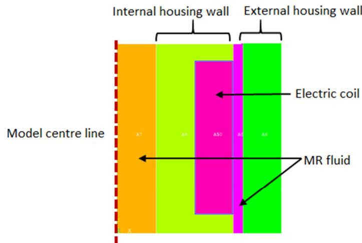
Fig. 2. 2D axisymmetric model of MR control valve
