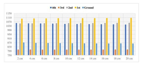
Fig. 13. Discomfort Hours using Vermiculite cement
