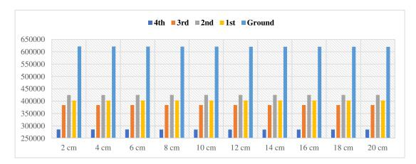
Fig. 6. Energy Consumption Using Extruded Polystyrene
