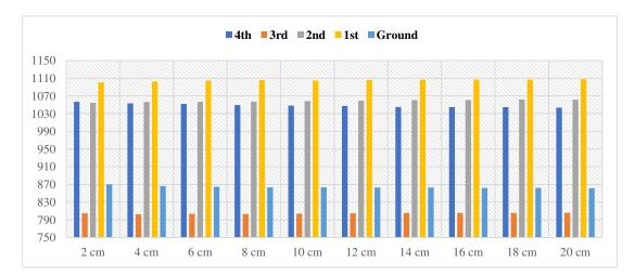
Fig. 7. Discomfort Hours using Polyurethane (0.045)
