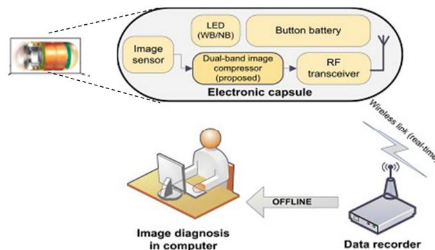
Fig. 1. Schematic diagram of wireless capsule endoscopy system [4]
