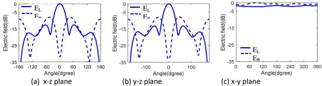
**Fig.6.** The circular polarization radiation patterns of the capsule module embedded in the human body model at 2.4 GHz in different planes
