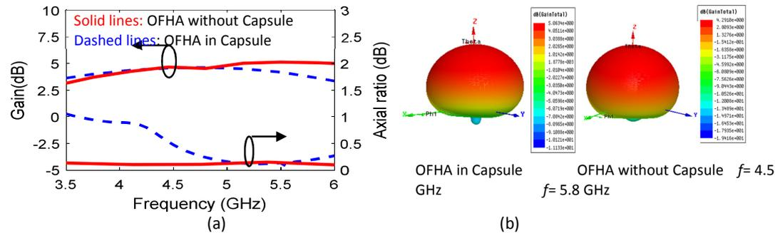
**Fig. 8(a).** The gain and axial ratio versus frequency (b) 3-D gain patterns at the resonance frequencies of the OFHA in capsule module and without capsule
