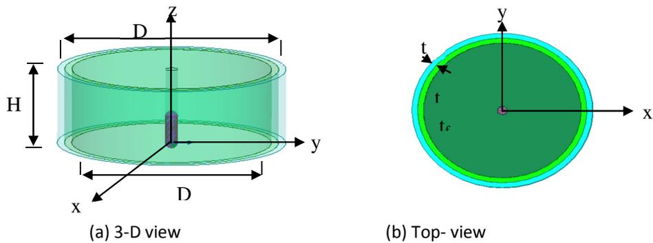
**Fig. 3.** The structure of multi-layered cylindrical body module with embedded capsule
