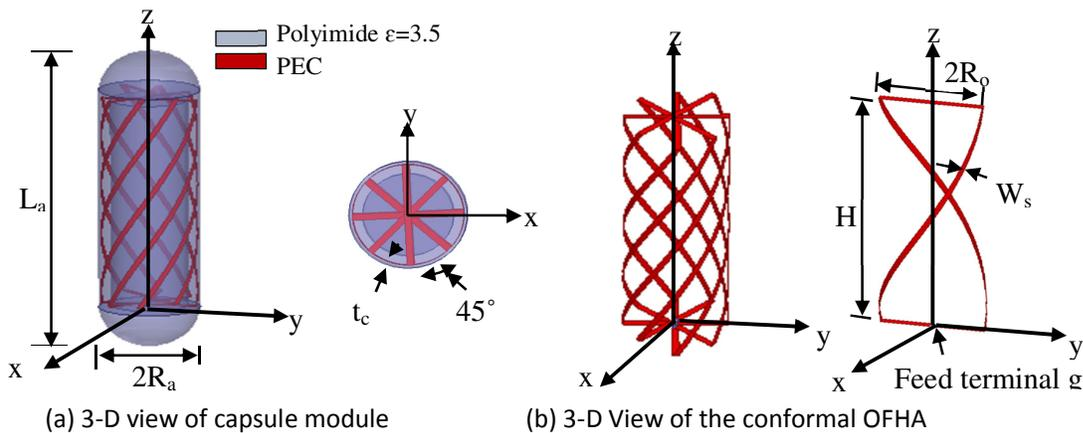
**Fig. 4.** The detailed construction of the capsule model with OFHA on its surface
