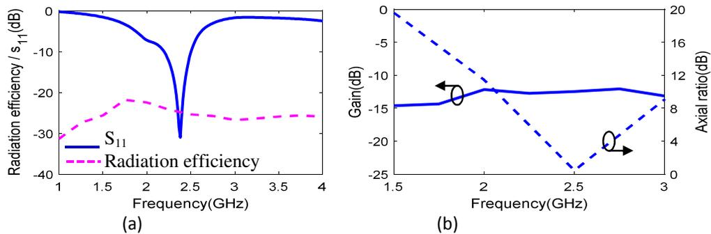
**Fig. 5.** (a) The reflection coefficient and radiation efficiency responses, (b) The gain and axial ratio responses of the capsule module embedded in the human body model
