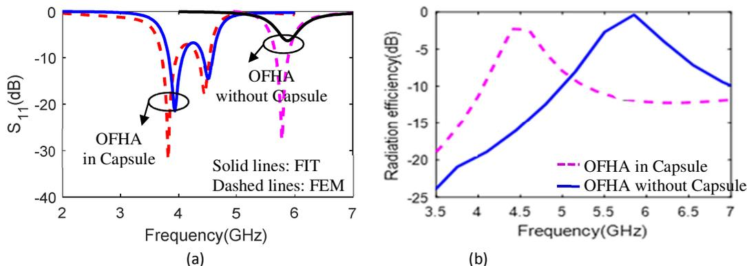
**Fig. 7.** (a) The reflection coefficient, (b) The radiation efficiency responses of the OFHA in capsule module and without capsule.
