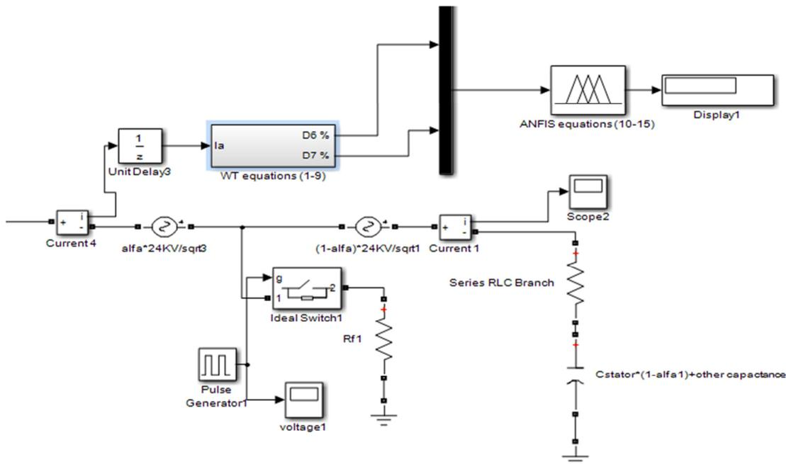
**Fig. 2.** Analysis of generator phase (A) current using Simulink model
