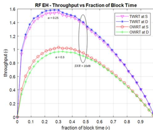
**Fig. 3.** Throughput vs EH Ratio at Destination Node with respect to Fraction of Block Time,  $\alpha$  for TSR Scheme, SNR=20dB
