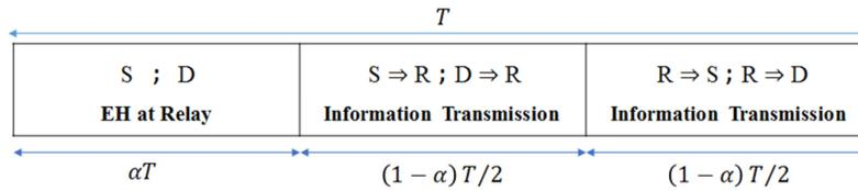
**Fig. 2.** Transmission Block Structure in TSR Scheme for EH and Information Transmission
