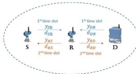
**Fig. 1.** Schematic Diagram for 3-Node with Two-Way Relaying
