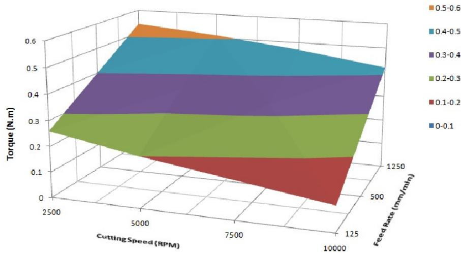
**Figure 6(b):** Effect of drill feed rate and cutting speed on torque.
