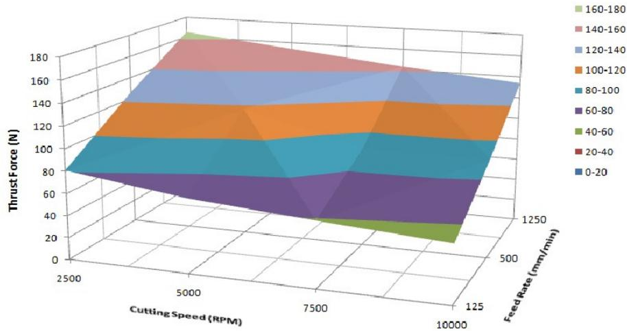
**Figure 6(a):** Effect of drill feed rate and cutting speed on thrust force.
