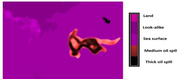
**Figure 5:** E-MMGA solution for oil spill discrimination in Scan Narrow beam SCNB data.
