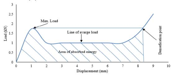
Fig. 5. Shows the area of absorbed energy in load-displacement curve [27]
