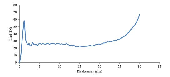
Fig. 8. Load-displacement curve for core cell size 20x40 mm
