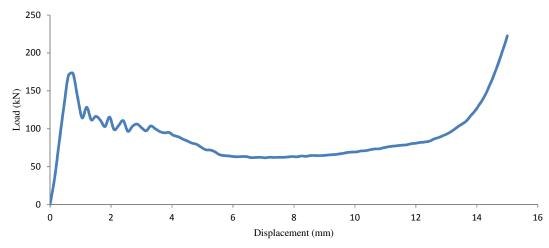
Fig. 11. Load-displacement curve for core cell size 50x20 mm
