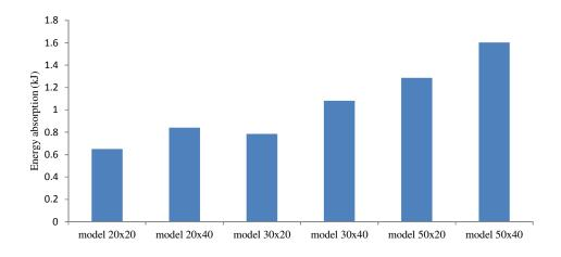
Fig. 13. Values of energy absorption for the models of study
