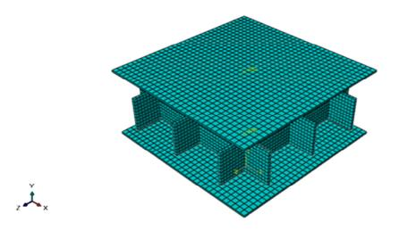
Fig. 1. Meshing of interlocking structure and platens
