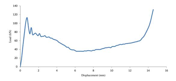
Fig. 9. Load-displacement curve for core cell size 30x20 mm
