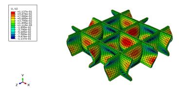
Fig. 6. the initial imperfection behavior of the model with size of 20x20 mm
