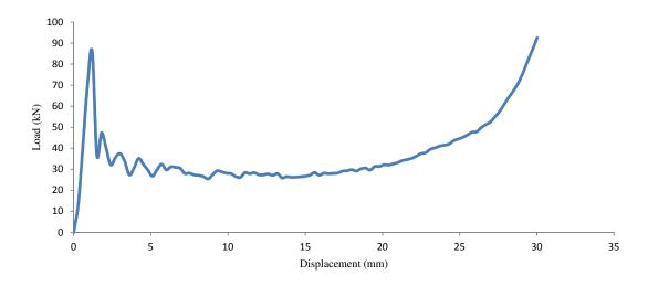
Fig. 10. Load-displacement curve for core cell size of 30x40 mm
