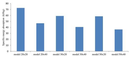
Fig. 14. Values of specific energy absorption for the models of study
