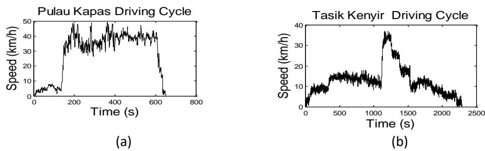
**Fig. 6.** The driving cycle used; (a) Pulau Kapas, (b) Tasik Kenyir
