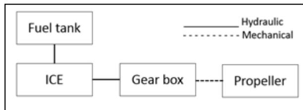
**Fig. 2.** Schematic illustration of conventional boat powertrain
