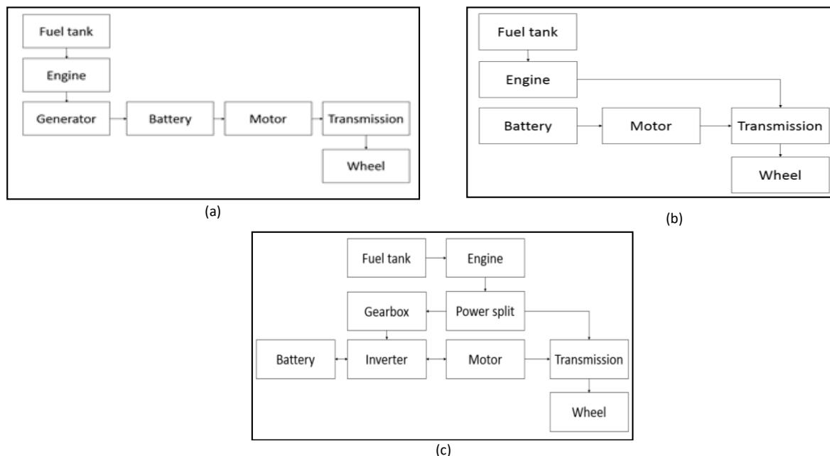
**Fig. 1.** The HEV drivetrain; (a) series hybrid, (b) parallel hybrid and (c)combined series-parallel hybrid
