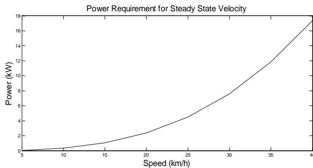
**Fig. 4.** Power Requirement for steady state velocity
