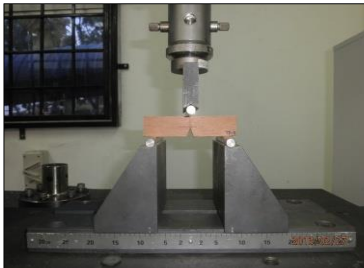
Fig. 2. Experimental Set-up for Fracture Toughness Test
