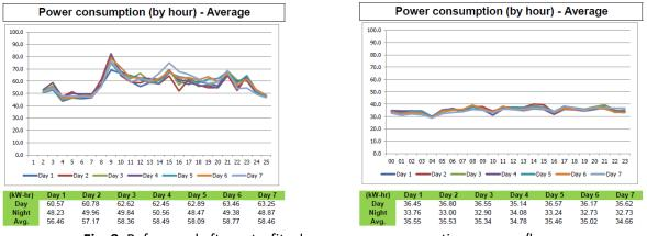
Fig. 8. Before and after retrofits doors power consumption average/hour
