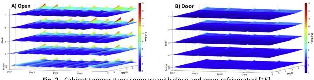
Fig. 2. Cabinet temperature compare with close and open refrigerated [15]
