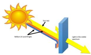
Fig. 3. Low-E filters on windows [21]
