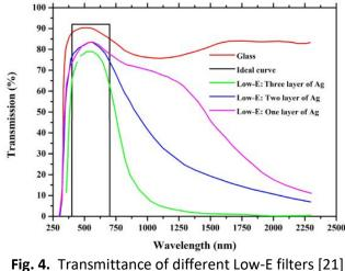
**Fig. 4.** Transmittance of different Low-E filters [21]
