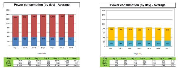
Fig. 7. Before and after retrofits doors power consumption average/day
