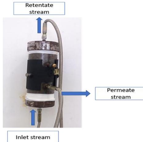
**Fig. 2.** Experimental set-up of membrane contactor separation process
