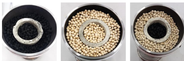
Fig. 2. The Type 1, 2 and 3 arrangements of adsorbent from left to right
