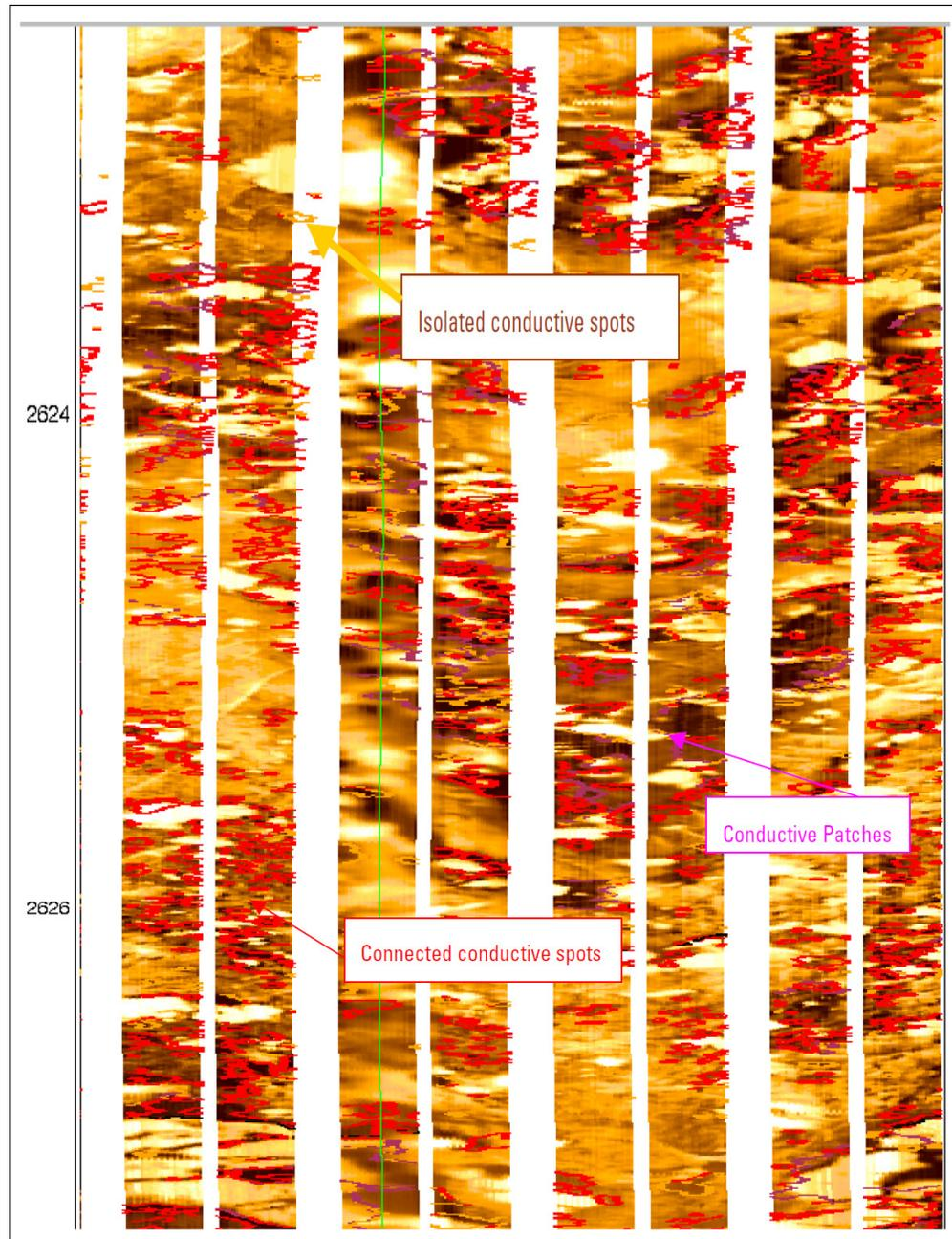
**Figure 4:** FMI calibrated images highlighting conductive features in a carbonate section. Contoured in red are conductive-connected spots (i.e. features smaller than  $0.0003 \text{ m}^2$ ); in dark brown are isolated conductive spots while dark magenta are conductive patches (i.e. conductive features larger than  $0.003 \text{ m}^2$ )
