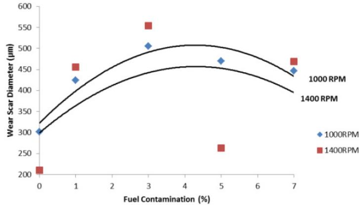
**Figure 6:** Graph of wear scar diameter [ $\mu\text{m}$ ] against fuel contamination [%]
