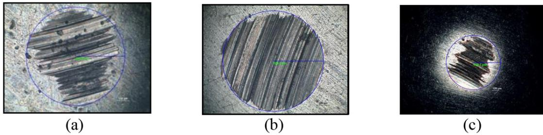
**Figure 8:** (a) Worn surface at 1000 RPM, 1% contamination; (b) Worn surface at 1400 RPM, 1% contamination; (c) Worn surface at 1000 RPM, 7% contamination
