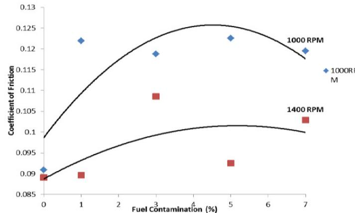
**Figure 5:** Graph of coefficient of friction against fuel contamination [%]
