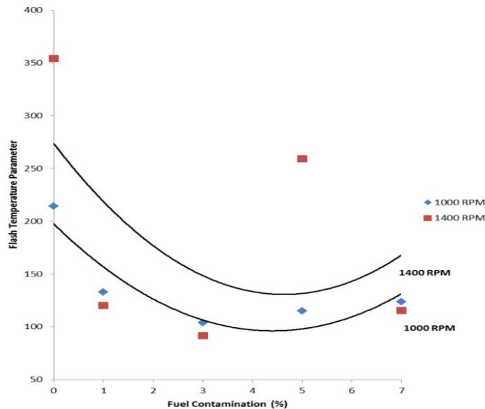
**Figure 7:** Graph of flash temperature parameter versus fuel contamination [%]
