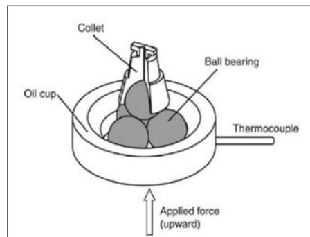
**Figure 2:** Schematic diagram of the Four Ball Tribotester assembly [5].
