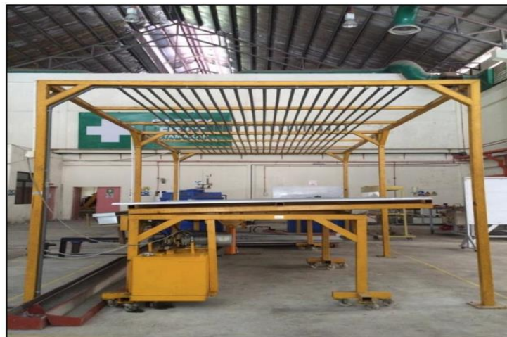
Fig. 4. Testing under a rainfall simulator
