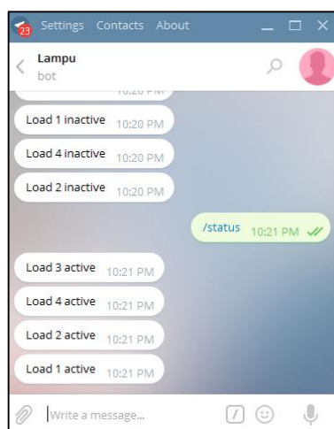
Fig. 7. Socket outlet status monitoring via Telegram apps
