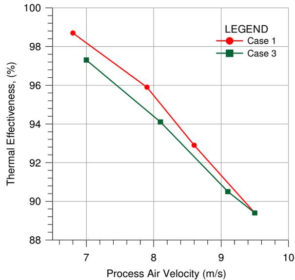
**Figure 3:** Effects of flow velocity of process air on thermal effectiveness.
