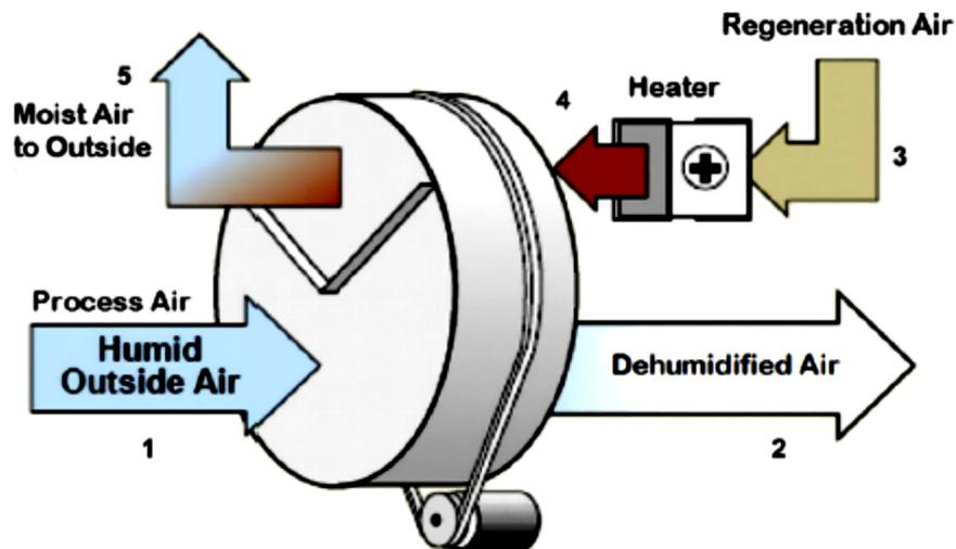
**Figure 2:** Schematic diagram of the dehumidifier unit [1].
