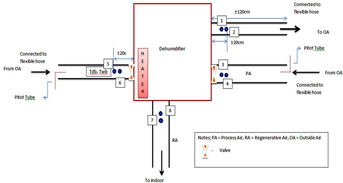
**Figure 1:** Schematic diagram of an air dehumidifier experimental apparatus.
