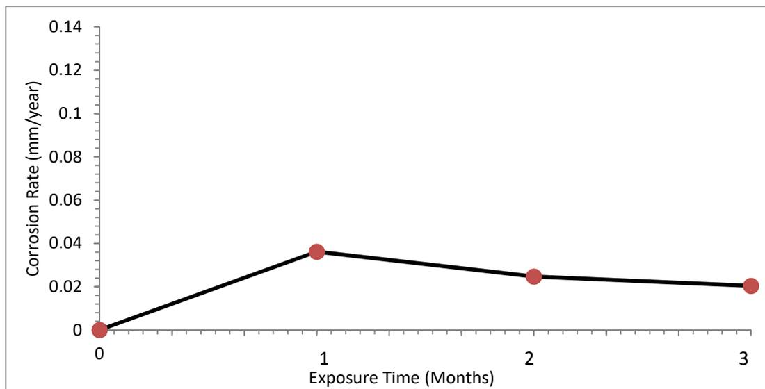
**Fig. 4.** Corrosion rate (mm/year) of samples for 1 to 3 months of exposure to 3.5 % NaCl solution.
