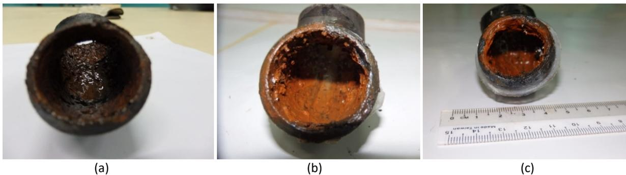
Fig. 2. Visual Inspection of the Surface and cross section of corroded samples (a) One month (b) Two months and (c) Three months exposure of the bends.
