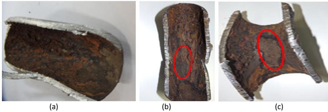
**Fig. 3.** Visual inspection after cleaning of smooth bend samples (a and b) inner diameter and (c) outer diameter.
