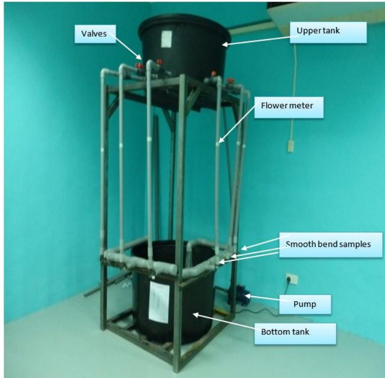
Fig. 1. Experimental set-up for flow-induced corrosion test.
