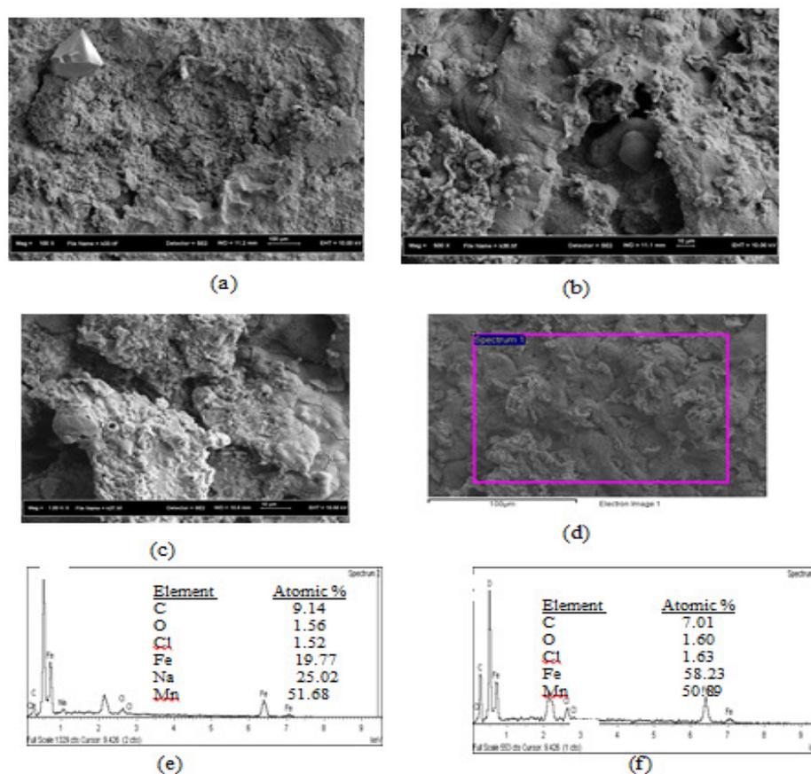
**Fig. 5.** FESEM and micro chemical composition of the corrosion product at the mitre elbow of 3.5% NaCl solution with different magnifications (a) 100x (b) 500x (c) 1000x (d) area of analysis - EDX (e and f) main compositions of the sample.
