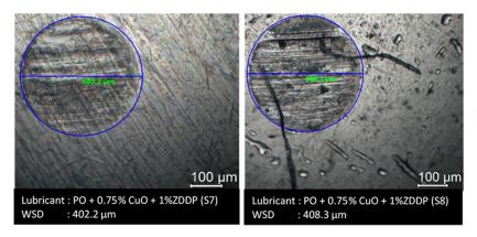
Fig. 3(d). WSD of S7 and S8 lubricants
