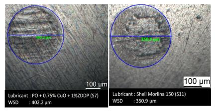
Fig. 3(f). WSD of S7 and mineral lubricants
