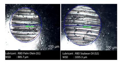
Fig. 3(a). WSD of S1 and S2 lubricants
