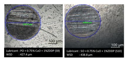
Fig. 3(e). WSD of S9 and S10 lubricants
