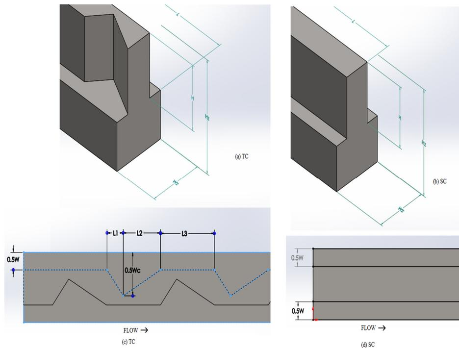
**Fig. 1.** Schematic diagram and geometry parameters of the microchannel: **(a)** schematic diagram of TC channel; **(b)** schematic diagram for SC channel; **(c)** geometry parameters of TC channel; **(d)** geometry parameters of SC channel
