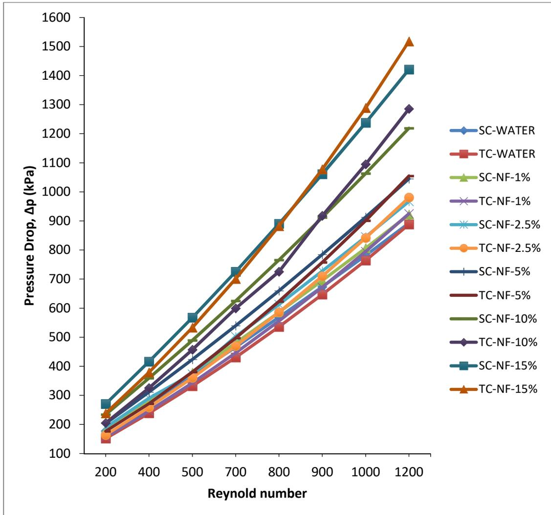
Fig. 3. Pressure drop of SC and TC vs varying Reynold number (Re)
