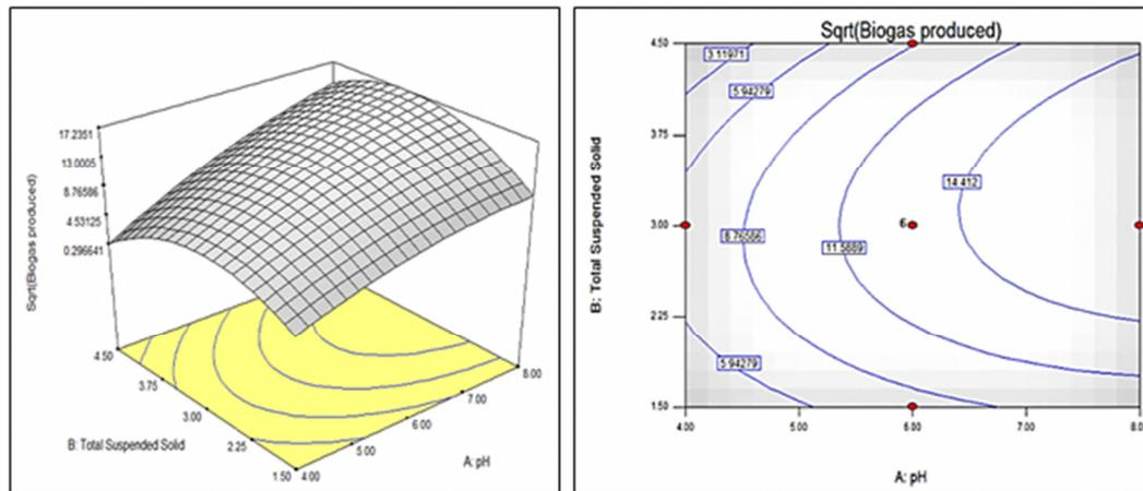
Fig. 4. Optimization of biogas with different variables: pH and TSS
