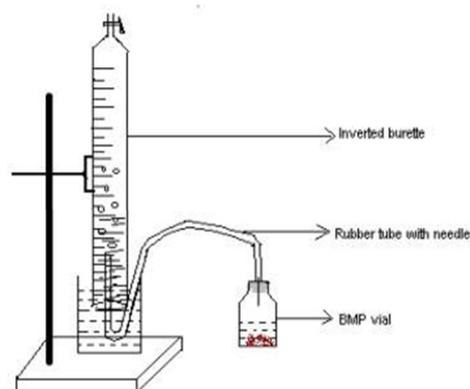
**Fig. 1.** Set up for water displacement method for biogas production
