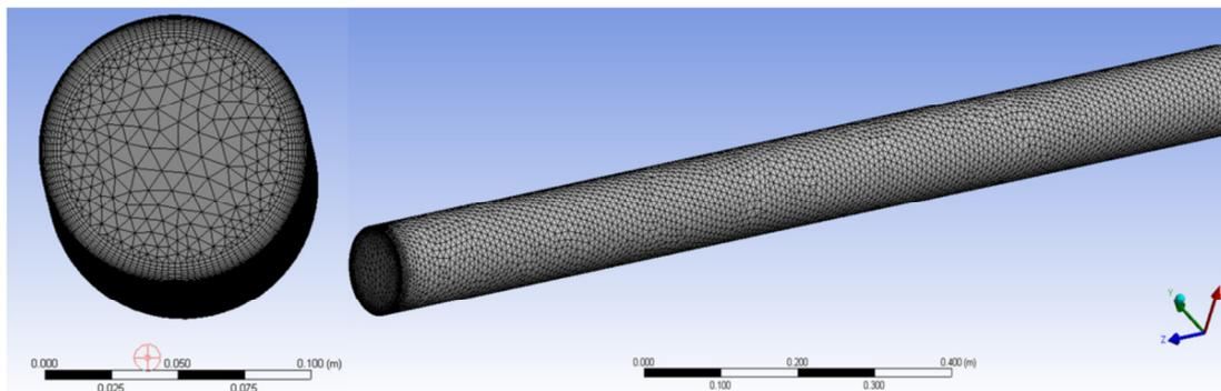
**Fig. 2.** The resulted tetrahedral mesh with inflation
