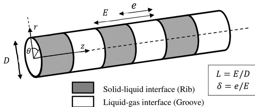
**Fig. 1.** Schematic diagram depicting flow in tubes having transverse superhydrophobic grooves
