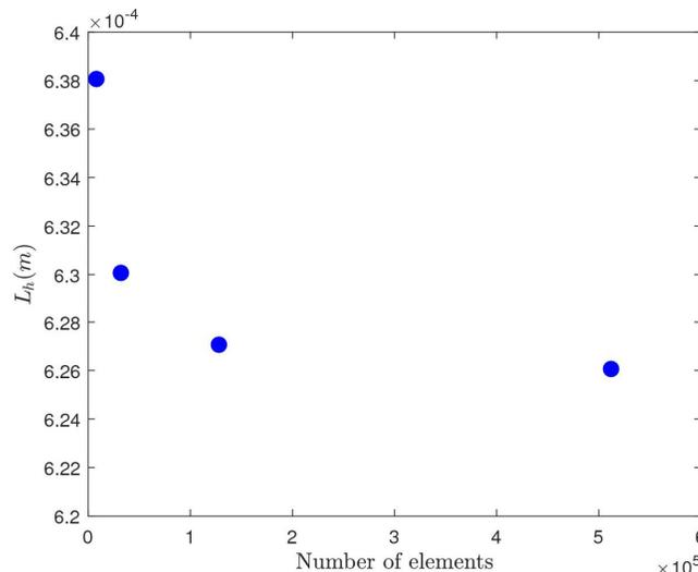
**Fig. 3.** Grid independence test for flow through pipe having transverse grooves with  $L = 0.1$  and  $\delta = 0.5$  at  $Re = 1$
