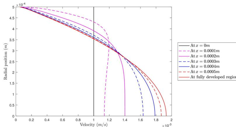
**Fig. 4.** Development of axial velocity along the pipe having transverse grooves of  $L = 0.1$  and  $\delta = 0.5$  at  $Re = 1$
