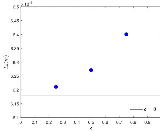
**Fig. 6.** Dependence of hydrodynamic entrance length on gas area fraction for flow over superhydrophobic transverse grooves of  $L = 0.1$  at  $Re = 1$
