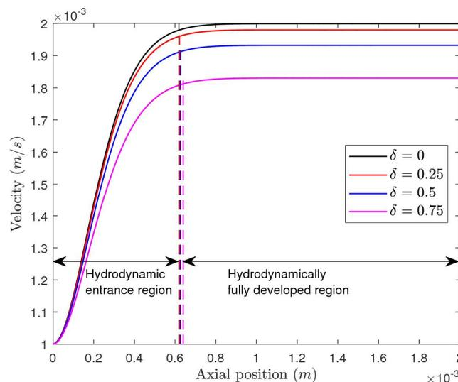
**Fig. 5.** Velocity magnitude along the centerline of the pipe for flow scenarios with  $\delta = 0, 0.25, 0.5$  and  $0.75$ . Simulations are conducted at  $Re = 1$  for  $L = 0.1$
