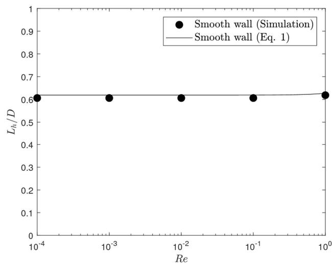
**Fig. 2.** Validation of numerical results of the normalized entrance length ( $L_h/D$ ) for different flow Reynolds numbers with correlation given in Eq. 1 by Durst *et al.*, [5]
