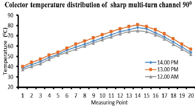
**Fig. 6.** Distribution of temperature along the channel with turn angle 90-degree for the time at 12 am – 2 pm.
