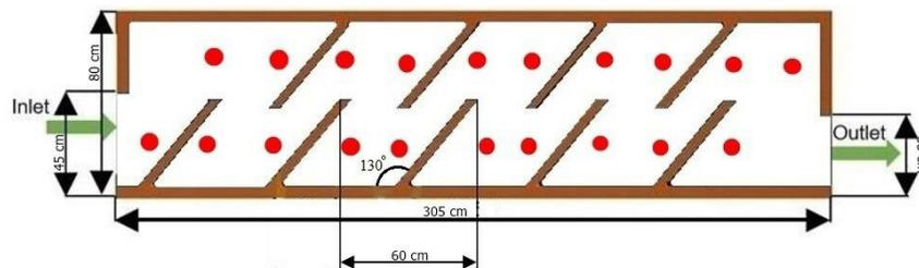
**Fig. 4.** Layout of obstacle and position of temperature measurement on sharp turn collector channel with 130-degree resistance angle
