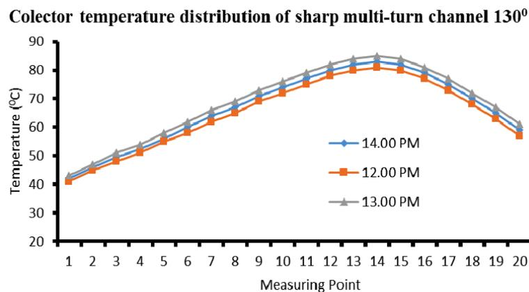
**Fig. 8.** Distribution of temperature along the channel with turn angle 130-degree for the time at 12 am– 2 pm
