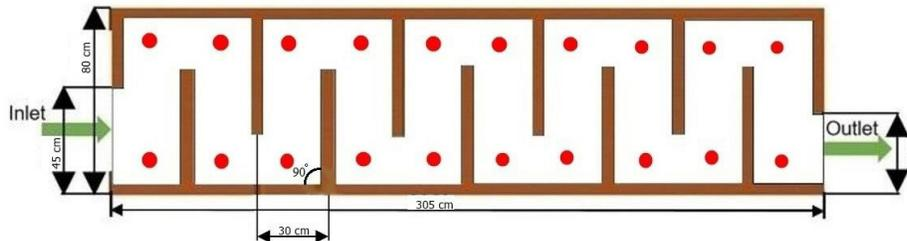
**Fig. 2.** Layout of obstacle and position of temperature measurement on sharp turn collector channel with 90-degree resistance angle
