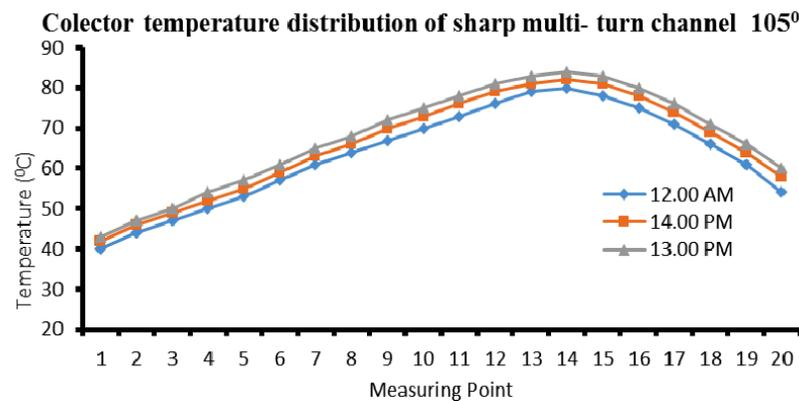
**Fig. 7.** Distribution of temperature along the channel with turn angle 105-degree for the time at 12 am-2 pm.
