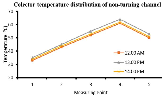
**Fig. 5.** Temperature distribution along the channel without obstacle with variation of measurement time
