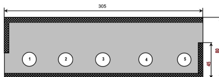
**Fig. 1.** The position of temperature measurement on the solar collector with a no - turning channel
