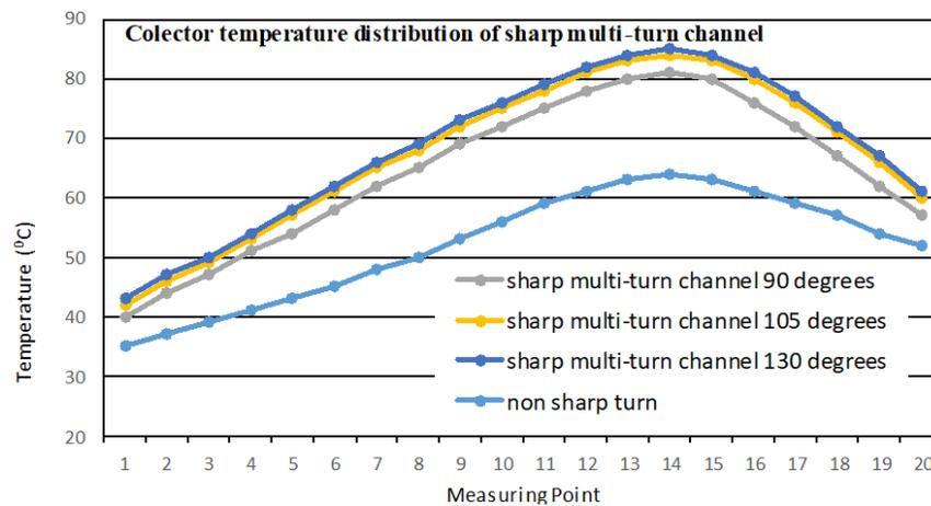
**Fig. 9.** Distribution of temperature along the channel with variations of passage
