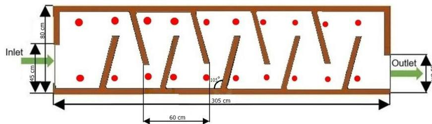
**Fig. 3.** Layout of obstacle and position of temperature measurement on sharp turn collector channel with 105-degree resistance angle
