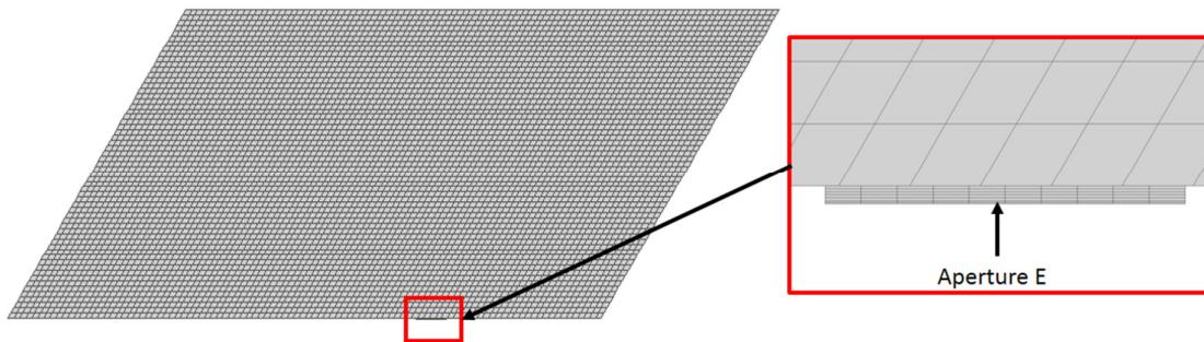
**Fig. 3.** Cross-section plane showing Aperture E location and mesh
