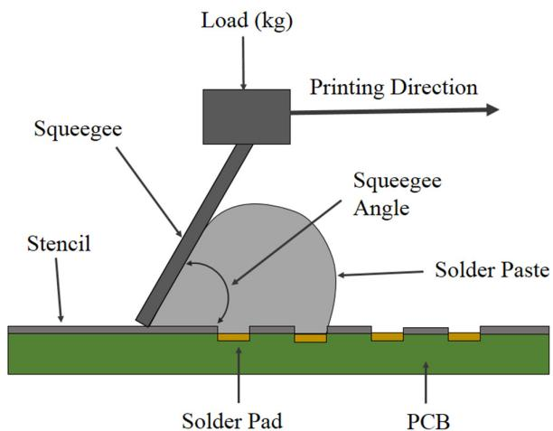
**Fig. 1.** Solder Paste Stencil Printing Process
