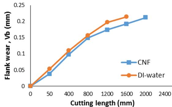
Fig. 2. Tool life of coated carbide insert under CNF nanofluid and deionized water
