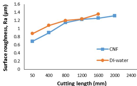
Fig. 3. Evolution of surface roughness for CNF nanofluid and deionized water
