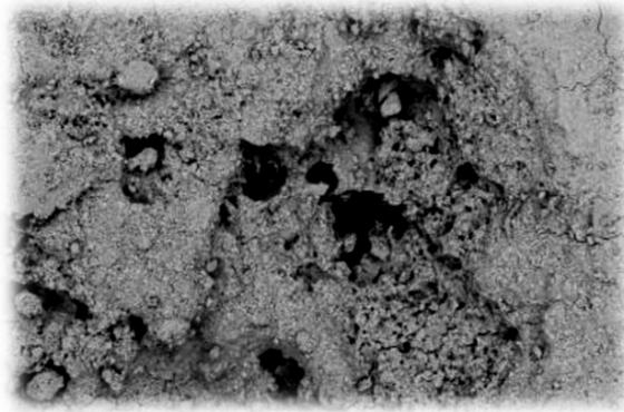
**Fig. 7.** Formation of voids in 950 kg/m<sup>3</sup> density with dominant void size of 0.55mm
