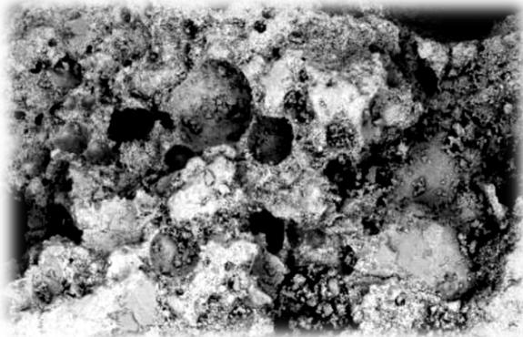
**Fig. 6.** Formation of voids in 750 kg/m<sup>3</sup> density with dominant void size of 0.66mm
