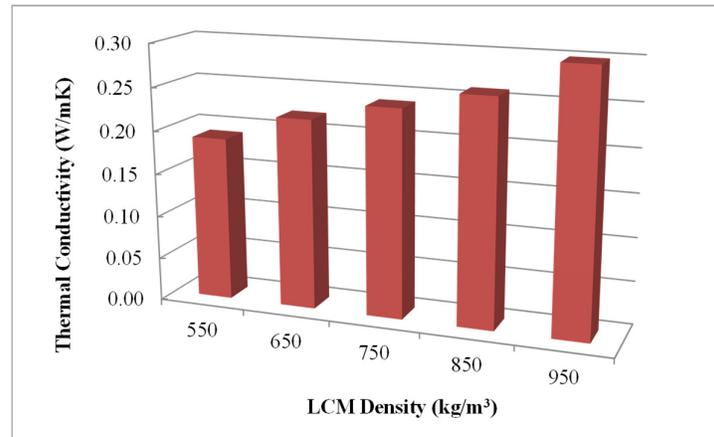
**Fig. 4.** Thermal conductivity of LCM of different densities
