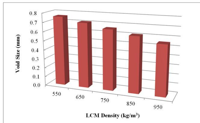
**Fig. 8.** Effective pore size of LCM at different densities
