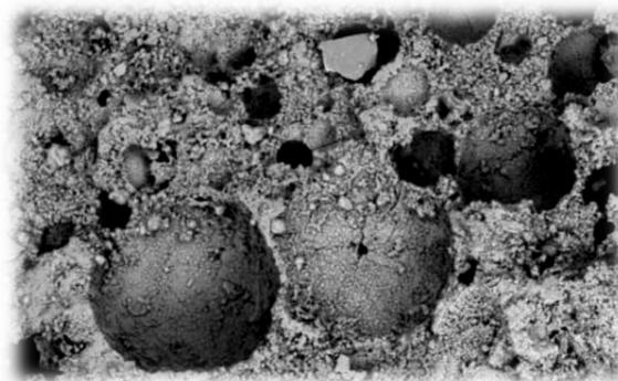
**Fig. 5.** Formation of voids in 550 kg/m<sup>3</sup> density with dominant void size of 0.76mm
