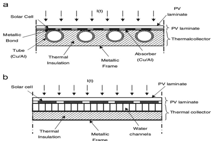
Fig. 2. Cross-sectional areas of Type A and B [12]
