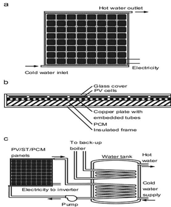
Fig. 2. Schematic model of PVT collector [7]
