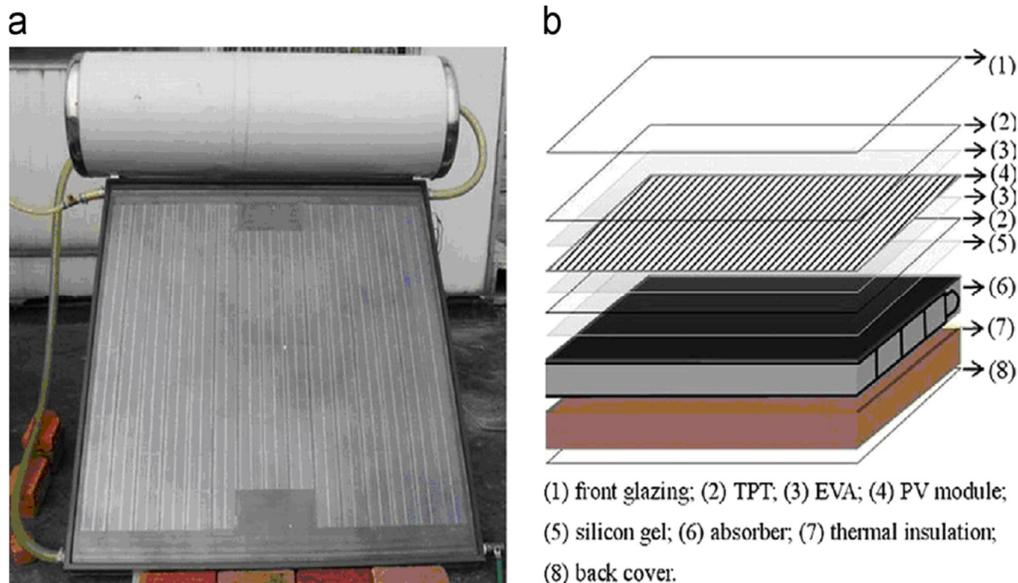
Fig. 4. The Hybrid PV water collector [16]
