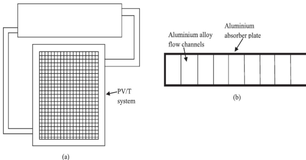
Fig. 5. (a) Front view of PV/T collector, (b) aluminium-alloy flow [37]
