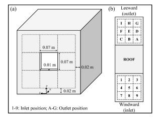
Fig. 2. Building model: (a) dimensions of opening; (b) possible locations of opening
