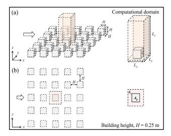
**Fig. 1.** Computational domain: (a) schematic view; (b) plan view
