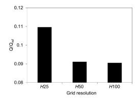
**Fig. 7.** Normalized ventilation rates for different grid resolutions
