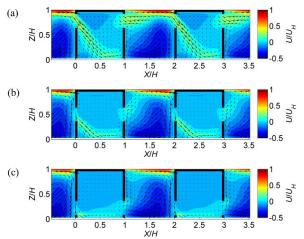
**Fig. 8.** Velocity contours and vectors for three different opening configurations: (a)2B; (b) 5E; (c) 8H
