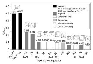
Fig. 14. Ranking of ventilation rate
