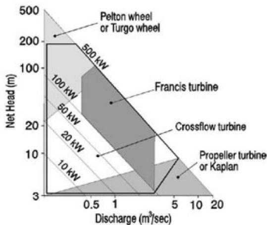
**Fig. 4.** Turbine Selection Based on Head and Flow Rate [16]
