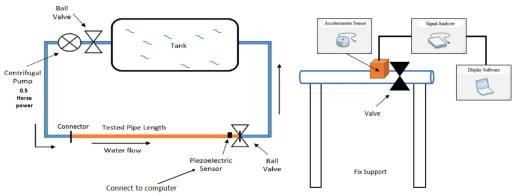
Fig. 4. Schematic Diagram [3]
