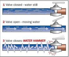
Fig. 1. Analogy water hammer [1]
