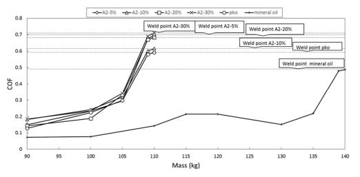
Fig. 5. Comparison of the coefficient of friction under extreme pressure
