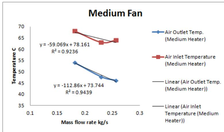
(b) Medium speed of fan in medium effects of heating
