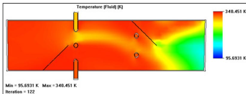
Fig. 15. Heat flow simulation of air as it exchanges heat with the fuel oil
