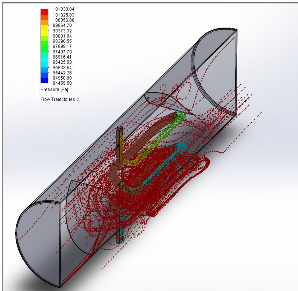
**Fig. 20.** Isometric view of pressure trajectory lines as it conveys the pipe and crosses the serpentine coil
