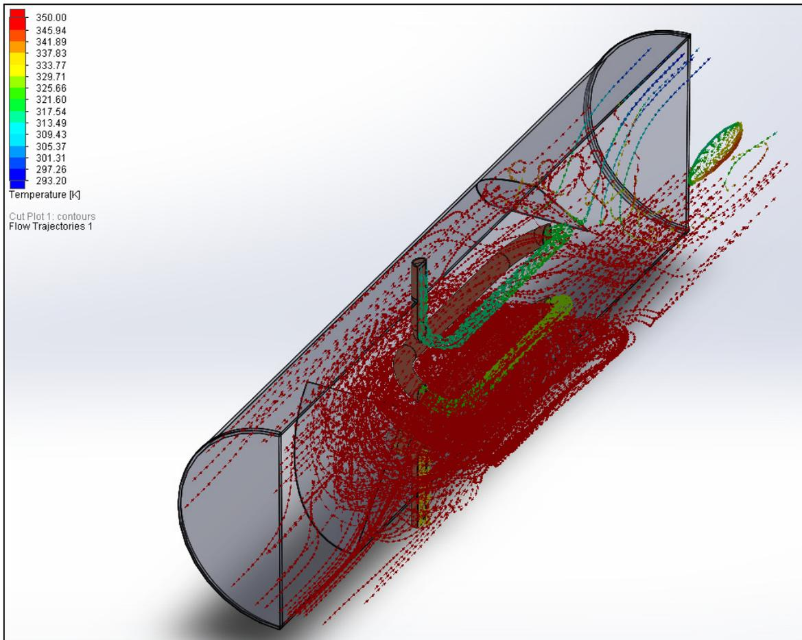
**Fig. 16.** Isometric view of air's heat flow trajectory as it exchanges heat with the fuel oil
