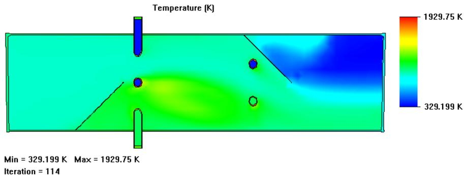
**Fig. 21.** Heat flow simulation of exhaust gas as it exchanges heat with the fuel oil
