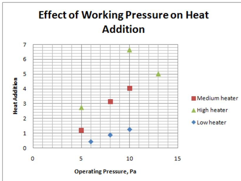
Fig. 13. Operating Pressure and heat addition relation
