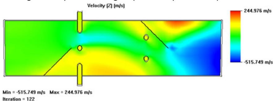
**Fig. 17.** Velocity distribution inside the conveying pipe as it surrounds the serpentine coil
