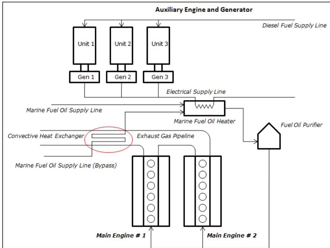
**Fig. 1.** Process flow and schematic diagram of heat exchanger set-up inside the vessel engine
