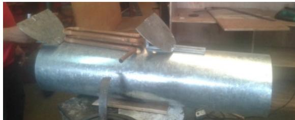
**Fig. 6.** Fabricated heat exchanger assembly, baffles, serpentine coil housing
