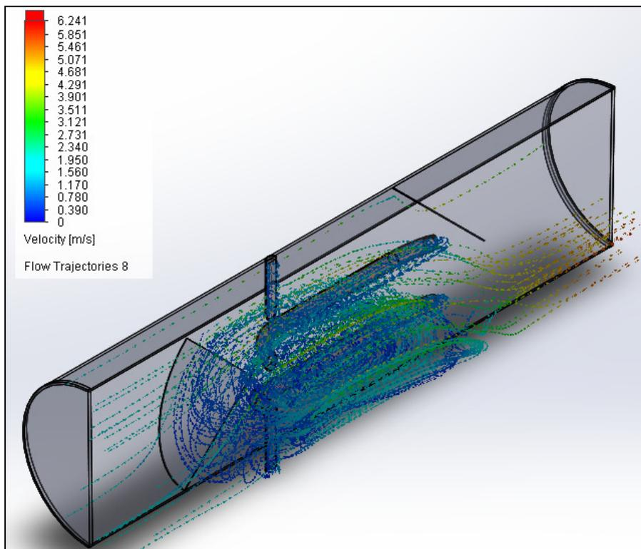
**Fig. 24.** Isometric view of velocity flow trajectory as it passes the serpentine coil heat where the fluid to be heated flows
