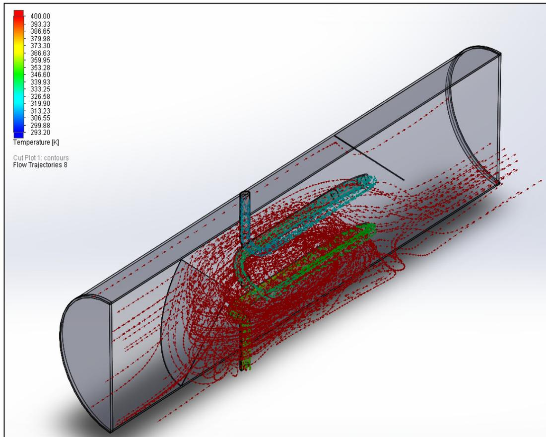
**Fig. 22.** Isometric view of exhaust gas heat flow trajectory as it exchanges heat with the fuel oil
