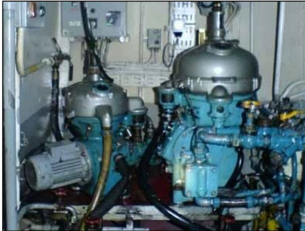
**Fig. 2.** Marine fuel preheating and purification system
