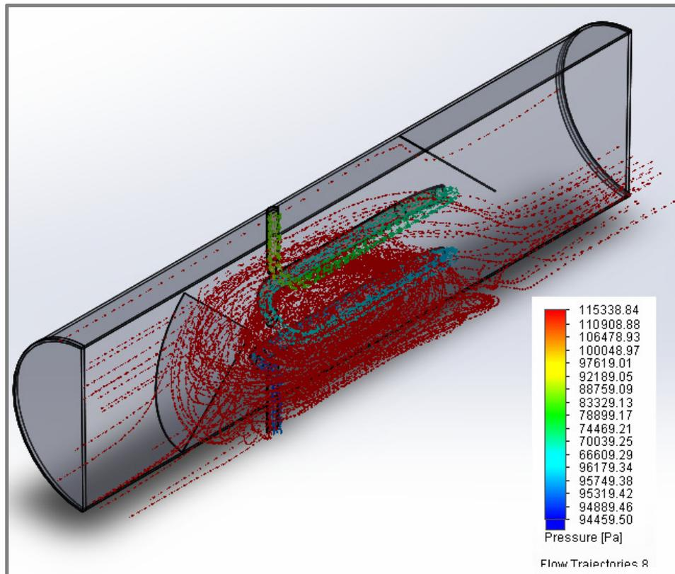
**Fig. 26.** Isometric view of pressure trajectory lines as it conveys the through the pipe crossing the serpentine coil
