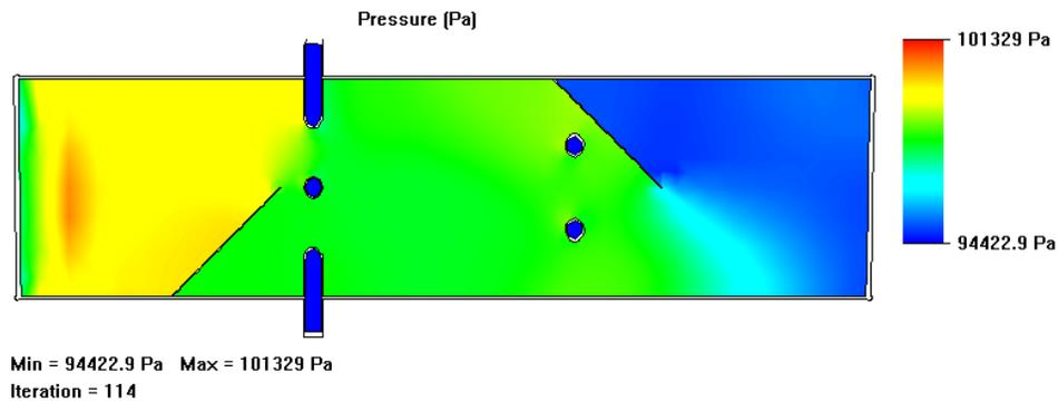
**Fig. 25.** Pressure distribution as air flows through the conveying pipe
