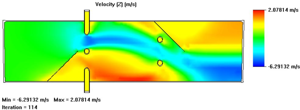
**Fig. 23.** Velocity distribution inside the conveying pipe as it surrounds the serpentine coil
