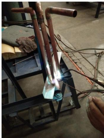
**Fig. 5.** Fabrication of serpentine copper tubing
