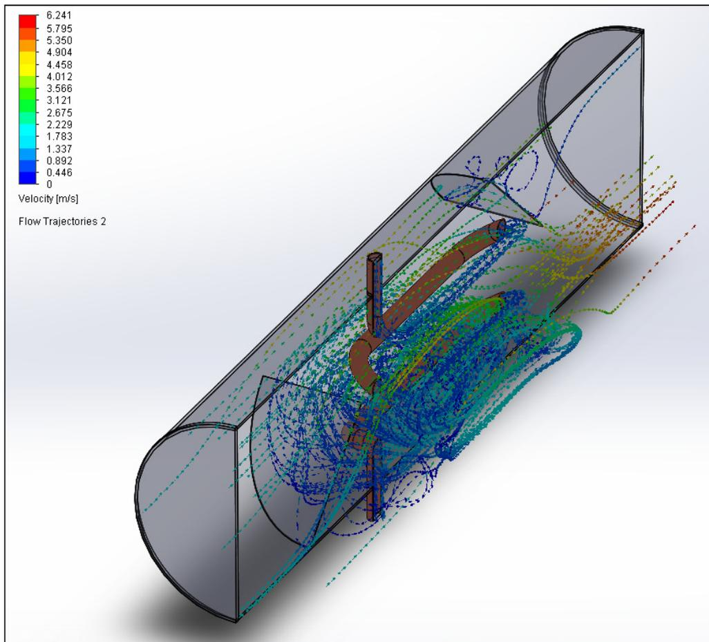
**Fig. 18.** Isometric view of velocity flow trajectory as it passes the serpentine coil heat where the fluid to be heated flows
