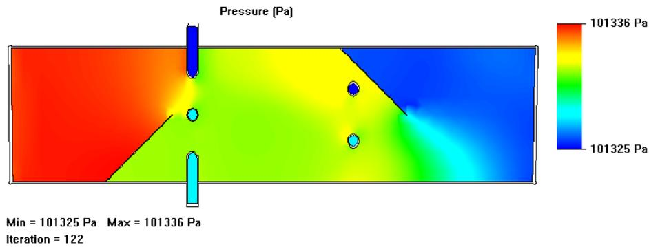
**Fig. 19.** Pressure distribution as air flows through the conveying pipe
