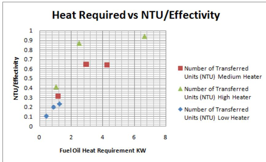
Fig. 14. Heat requirement of Fuel Oil with respect to heat transfer effectivity
