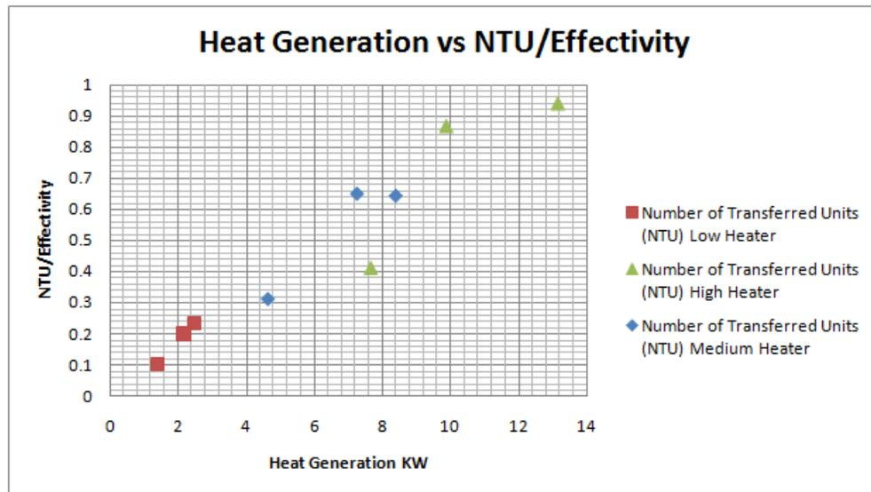
**Fig. 11.** Effectivity of heat transfer per heat generation
