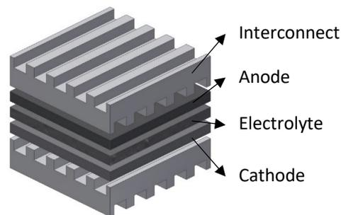
**Fig. 2.** Schematic of SOFC planar design
