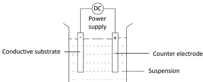
Fig. 4. Schematic of cathodic EPD set up
