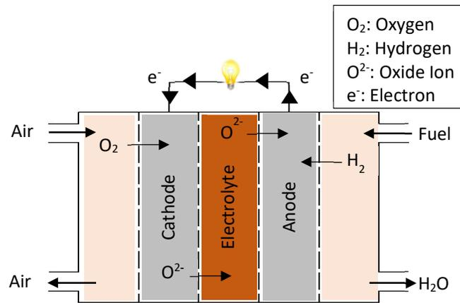
**Fig. 1.** Schematic of SOFC operation and components
