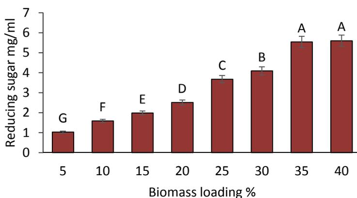
**Fig. 4.** Effect biomass loading on the obtained reducing sugar in IL-E hydrolysis system ( $R^2=0.9958$ )
