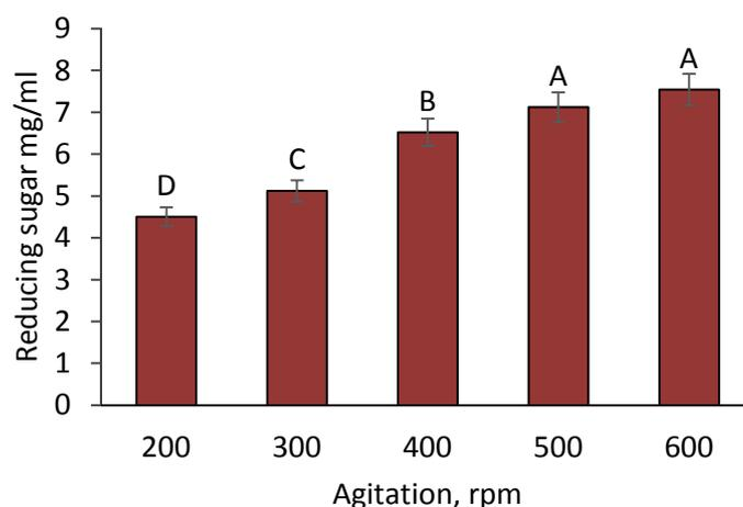
**Fig. 6.** Effect of agitation on the obtained reducing sugar in IL-E hydrolysis system ( $R^2 = 0.9898$ )
