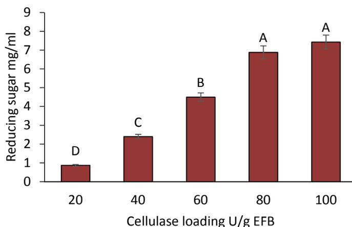
**Fig. 5.** Effect of cellulase loading on the obtained reducing sugar in IL-E hydrolysis system ( $R^2 = 0.9898$ )
