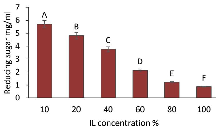
**Fig. 3.** Effect of IL concentration on the obtained reducing sugar in IL-E hydrolysis system ( $R^2 = 0.9927$ )
