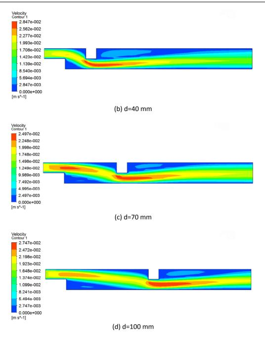
Fig. 8. Velocity contour for all studied geometry
