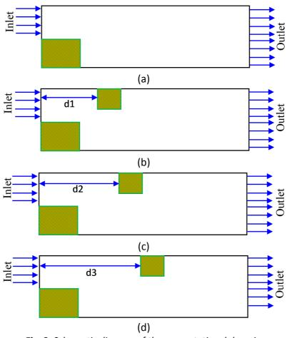
Fig. 2. Schematic diagram of the computational domain
