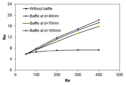
Fig. 6. Average Nusslet number of the channel with and without baffle
