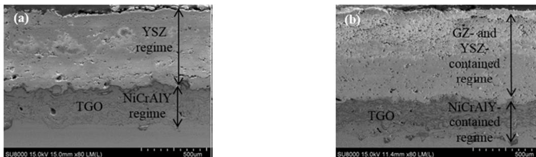
**Fig. 3.** Micrographs of the oxidised samples of (a) typical YSZ system, and (b) GZ/YSZ system
