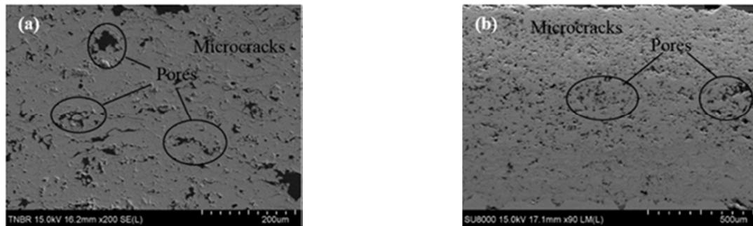
**Fig. 2.** Micrographs of the as-sprayed samples of (a) typical YSZ system, and (b) GZ/YSZ system
