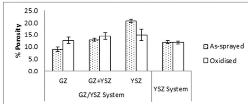
**Fig. 4.** Measurement of porosity on both samples in as-sprayed and oxidised conditions
