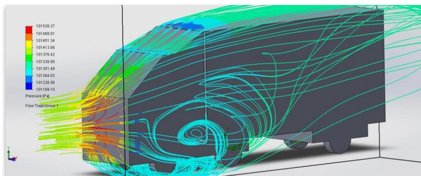
**Fig. 7.** Flow over the truck with cab-extender at  $25^\circ$
