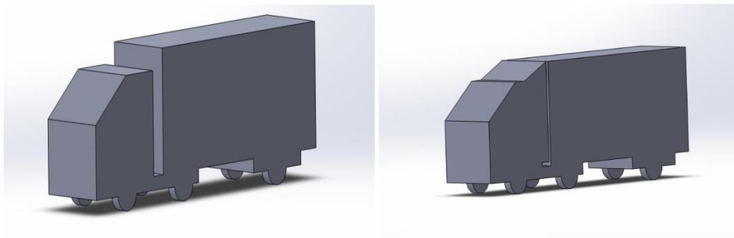
Fig. 1. Model with and without cab-extender
