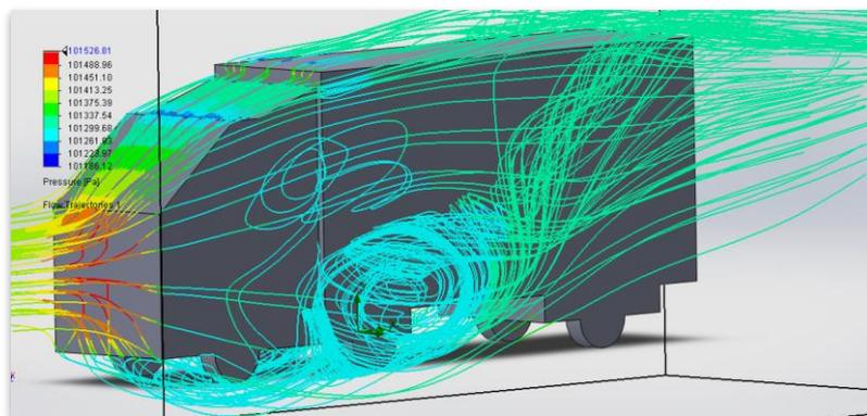
**Fig. 6.** Flow over the truck with cab-extender at  $10^\circ$
