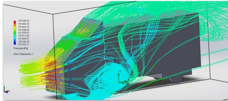
Fig. 8. Flow over the truck with cab-extender at 38°
