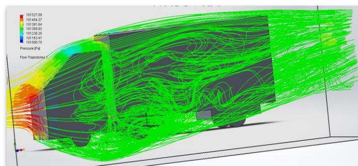
**Fig. 5.** Flow over the truck without cab-extender
