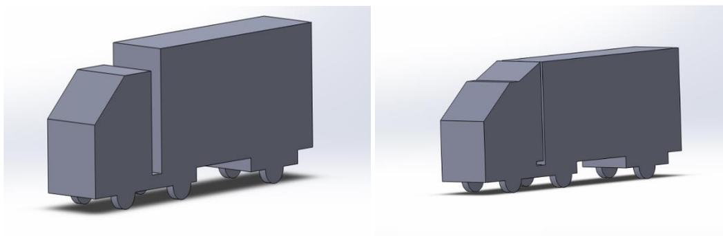
Fig. 1. Model with and without cab-extender
