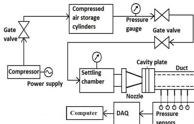
Fig. 3. Schematic description of experimental Setup
