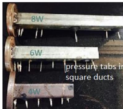
Fig. 5. Different L/W ratio ducts
