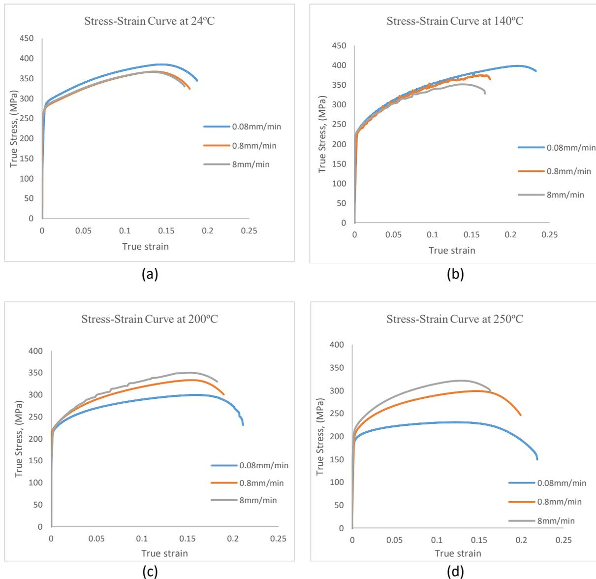
**Fig. 4.** (a-d) AA6061 Stress-Strain curves at different strain rates and temperature
