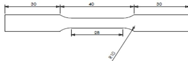
**Fig. 3.** Configuration ASTM E21
