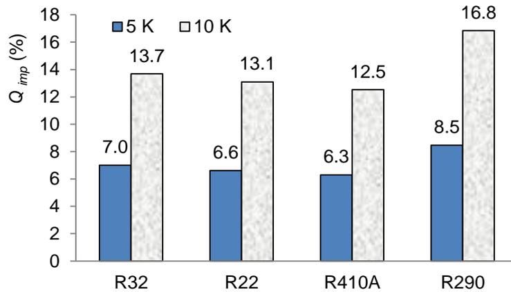
**Fig. 5.** The refrigerating effect improvement for four refrigerants
