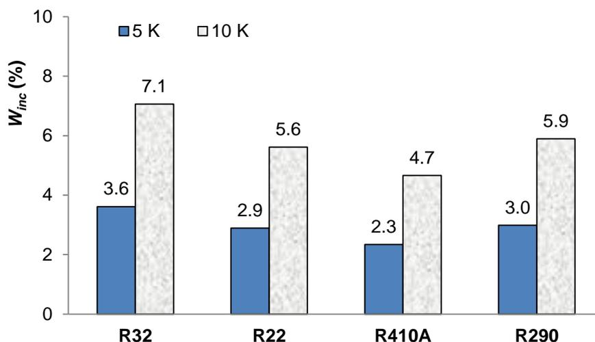
Fig. 7. The compressor input improvement for four refrigerants
