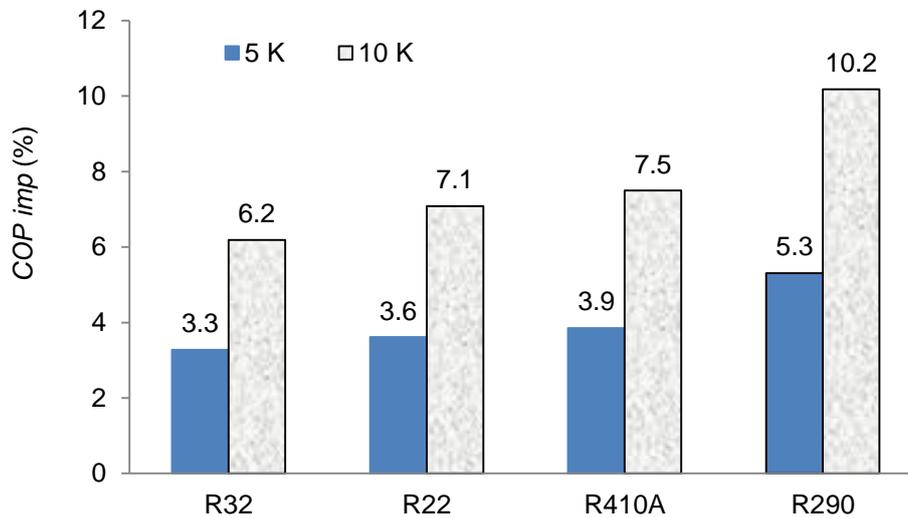
Fig. 9. The *COP* improvement for four refrigerants
