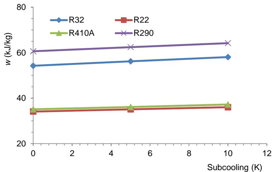
**Fig. 6.** The compressor work versus subcooling
