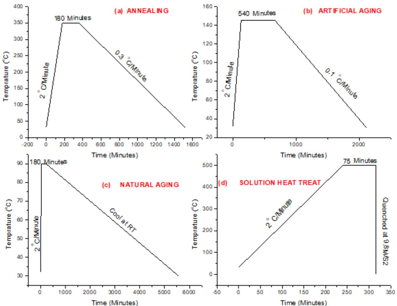
**Fig. 1.** Heat treatment profiles (a) annealing (b) artificial aging (c) natural aging (d) solution heat treatment quenched in clean water
