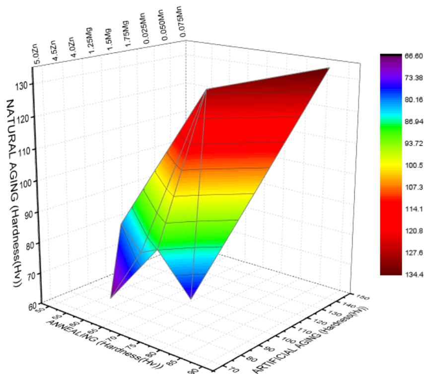
**Fig. 3.** Micro hardness of alloy compositions against T4, T6 and O heat treatments
