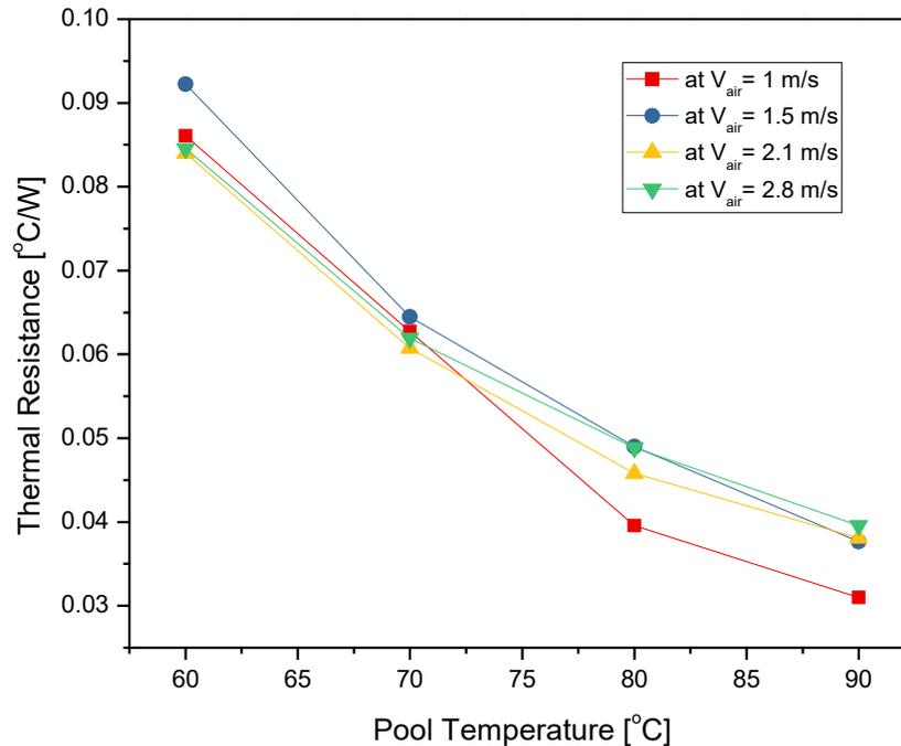
Fig. 4. Thermal resistance of vertical straight wickless-heat pipe
