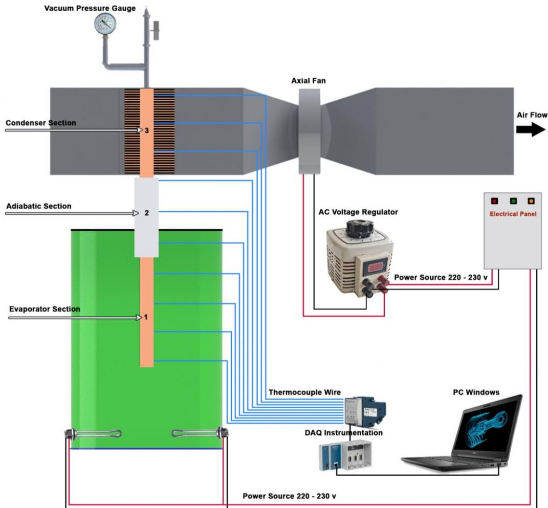
**Fig. 1.** Experimental setup of vertical straight wickless-heat pipe
