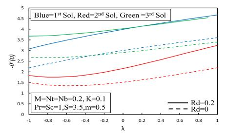
Fig. 5. Variation of heat transfer rate at various values of  $\lambda$  and Rd
