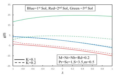
Fig. 4. Variation of couple stress coefficient at various values of  $\lambda$  and K
